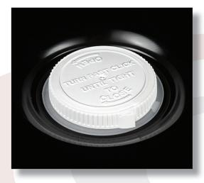
The Stolz closure was developed in conjunction with Rieke Packaging Systems, a leader in the closure industry, and is available exclusively through Cleveland Steel Container and approved distributors. The Stolz closure is a large 57mm all plastic fitting specifically designed for use in a steel pail cover. It is ideal for tinting, mixing and dispensing products. The cap is made from High Density Polyethylene.
